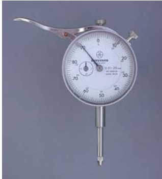
Gambar 5.7. Jam ukur ( Dial Indicator )
